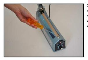
**Step I.** Remove the PTFE Cover. Loosen the screws that hold the PTFE cover plates on both sides of the sealer's body. It is not necessary to remove the screws completely. Lift the PTFE Cover to expose the heating element.
