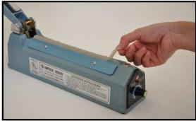
**Step 3.** Remove the PTFE Adhesive. Peel the PTFE Adhesive from the sealer's body.
